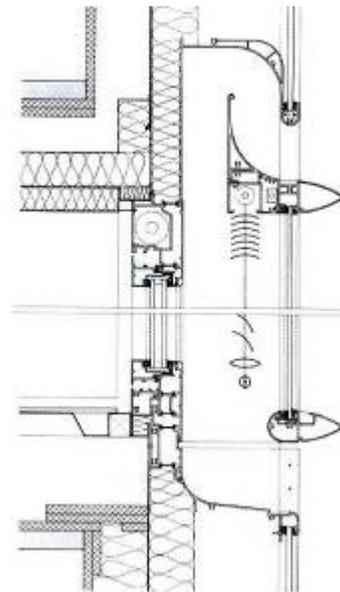
**Figure 3-49- details of opening windows in double layered facade. Source: BUCHANAN, 2005.**
