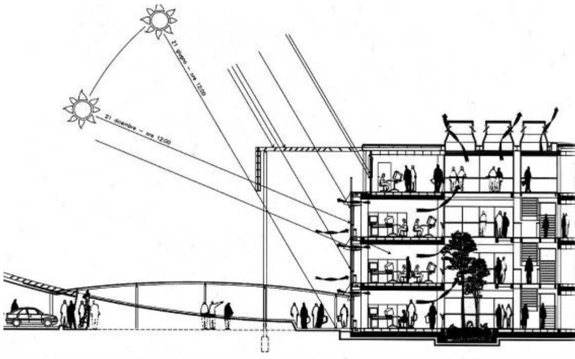
Figure 3-37- Cross section showing the shading and ventilation strategies.
