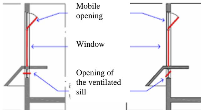
**Figure 3-19- Detail of the ventilated sill**
