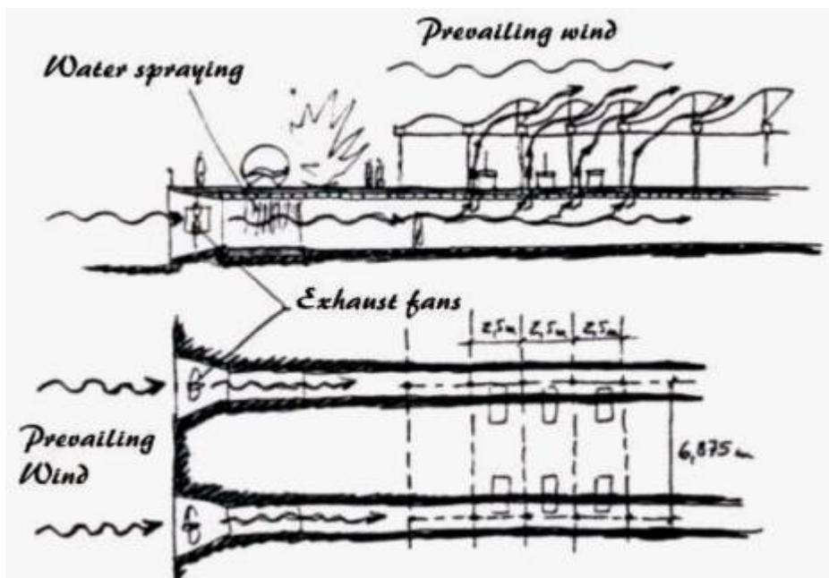
Figure 4-17 - Lele's sketches of the ventilation system of the hospital in Salvador. (LATORRACA, 2000)
