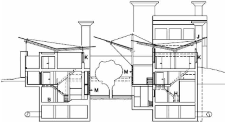
**Figure 3-58- Cross section of the hotel in India. Internal courtyard, overhangs and rooms partly underground.**
