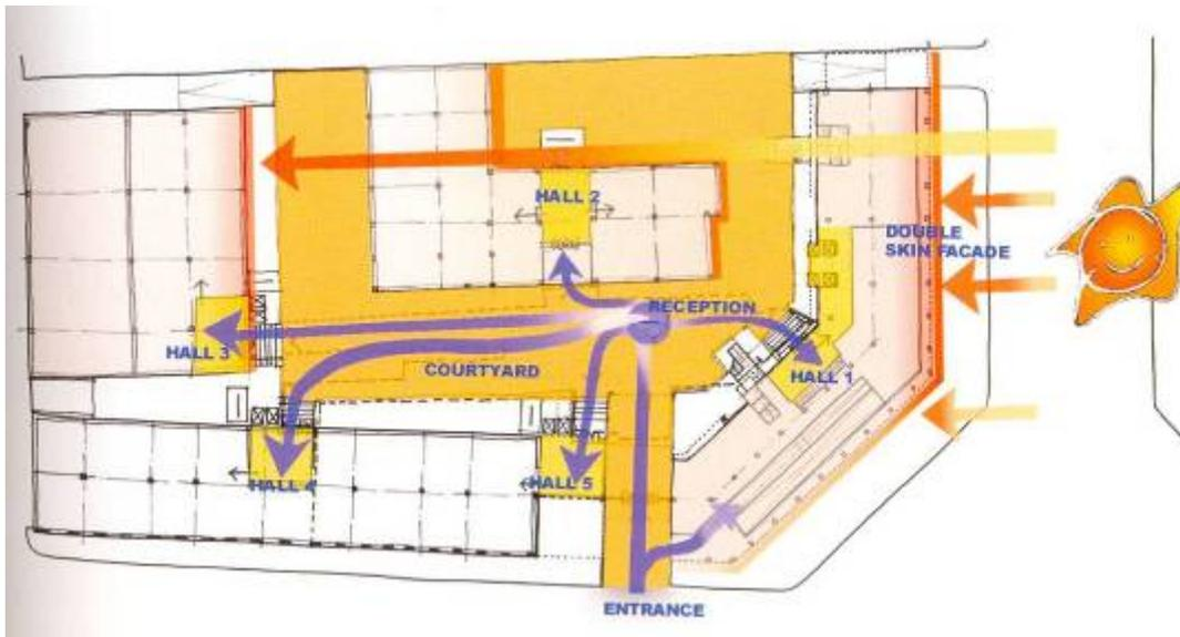
**Figure 4-19- Schematic Plan of the Milan Project. Cucinella, 2004.**
