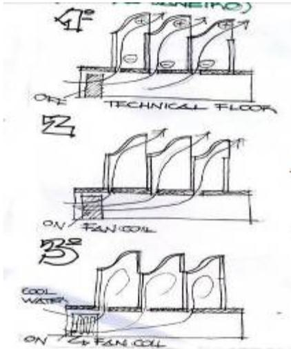
Figure 4-20- Sketches of the three different cooling systems in Rio de Janeiro's hospital.
