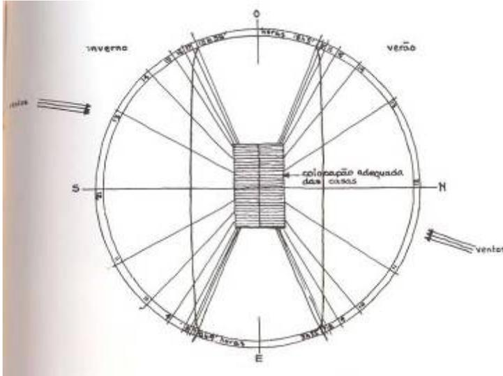
Figure 2-6 - Analysis of insolation, daylighting and ventilation. Source: (RIBEIRO, 1992)
