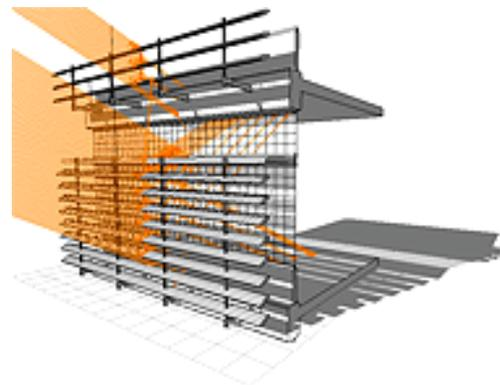
**Figure 3-62- Solar incidence on shading devices (www.squ1.com).**
