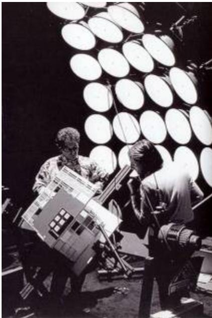
**Figure 4-22-** Use of artificial sky to analyze daylight effect on physical model. Source: Cucinella, 2004
