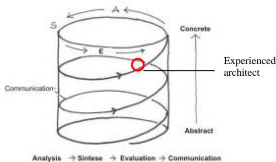
**Figure 4-8 Model of Asimow’s design process.**
