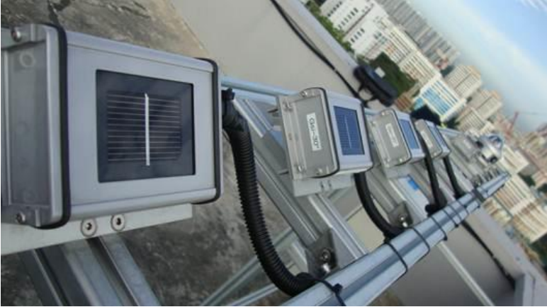
Figure 37: SERIS meteorological station rack, with tilted silicon sensors ranging from 0 to 40 degrees (source: SERIS).
