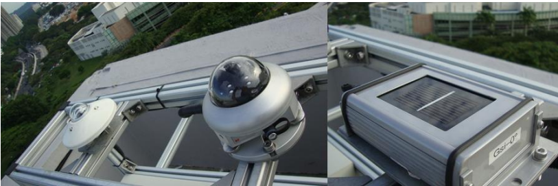
Figure 33: Three irradiance devices measuring global horizontal irradiance located at the SERIS meteorological station in Singapore (source: SERIS).
