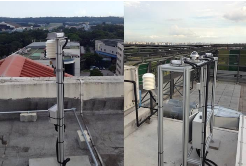
Figure 72: Basic meteorological station #425 (left) and superstation #408 (right, wind sensors not pictured) (source: SERIS).
