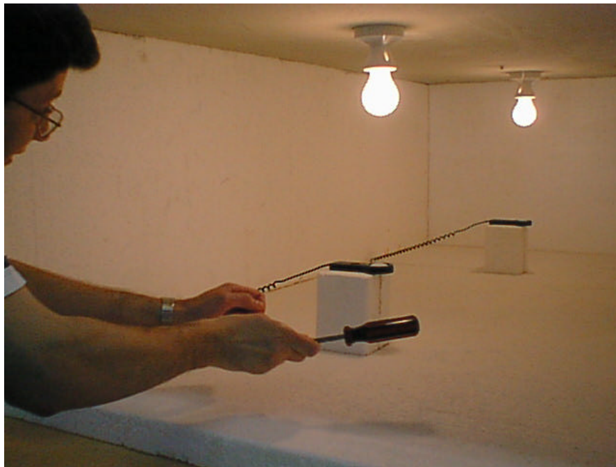
Figure 6.3. Light bulbs and photocells installed in the model.
