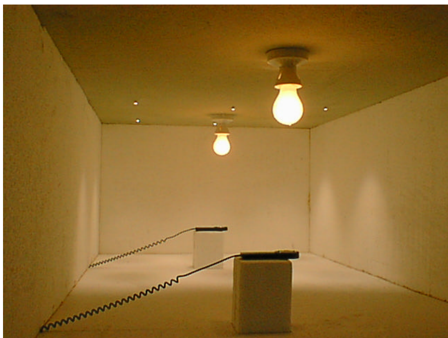
Figure 6.5. The fibre optic system and the light bulbs installed in the model.
