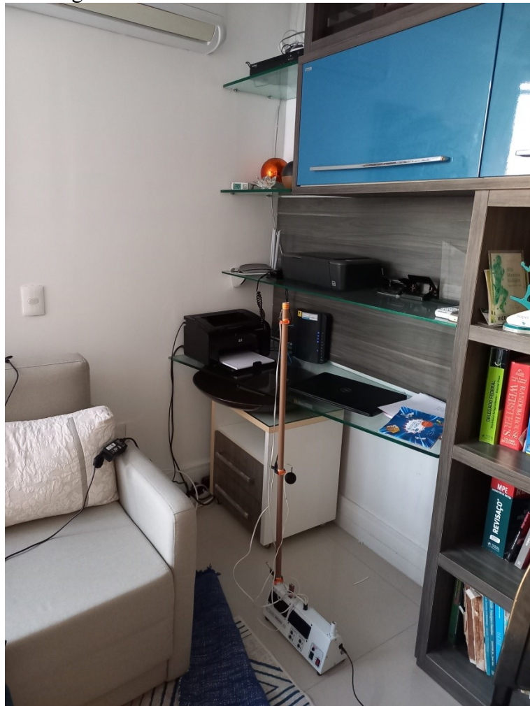
Figure 9 – Positioning of a SENSU microclimatic station for additional measurements
