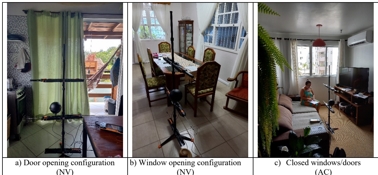
Figure C 6 – Illustration of the representative window/door configurations which would influence airflow distribution in residences
