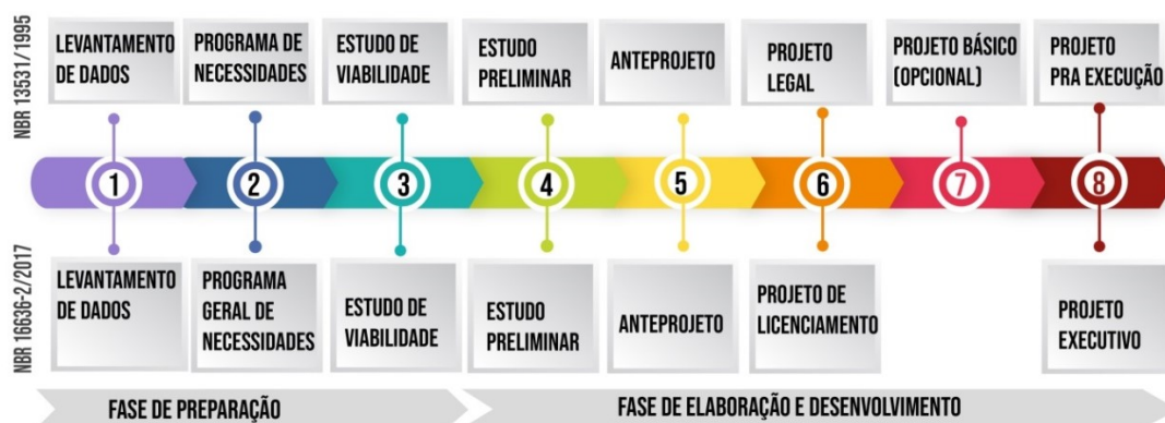
Figura 6: Fluxograma comparativo entre as normas NBR 13531/1995 e NBR 16636-2/2017
